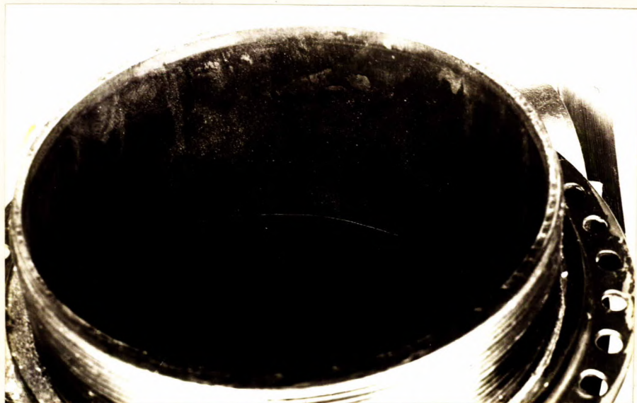
CRACK OUTLINED BY MAGNAFLUX POWDER. (Approximately 2/3 size).
