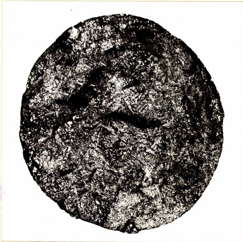
PHOTO SHOWING DENDRITES IN STEEL. (Approximately 4 times actual size).
