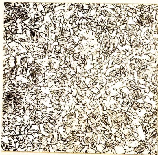
X500, nital etch. CORE OF PIN.
