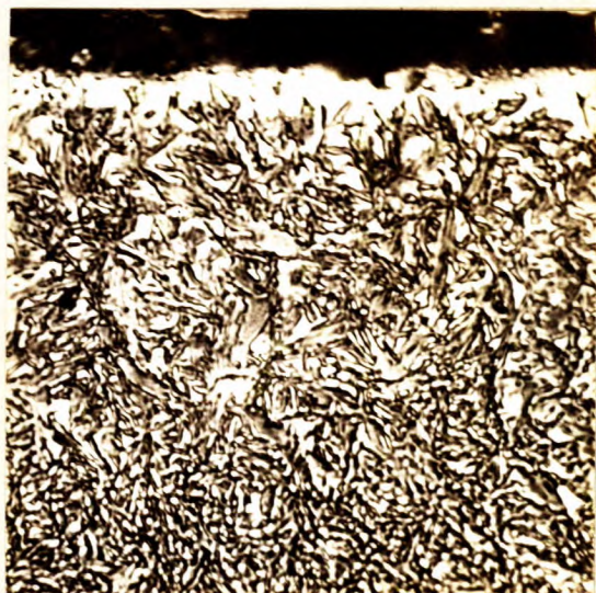
X1000, nital etch. CASE OF PIN.
