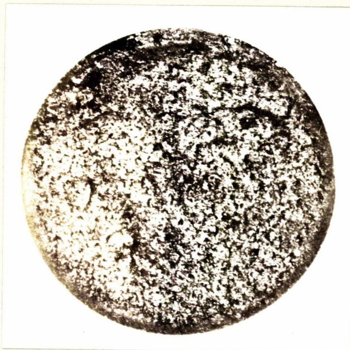
FRACTURED SURFACE OF PIN.
