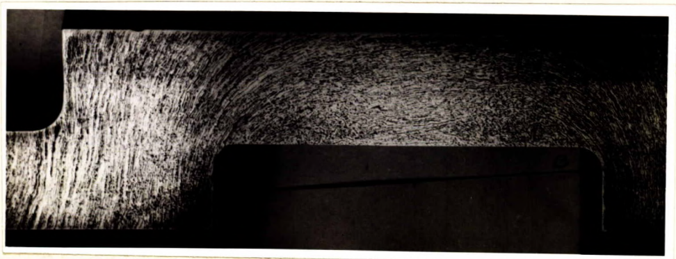
F LOW L INES N EAR F ILLET S IN UNDER SIDE OF CRANK PIN.
