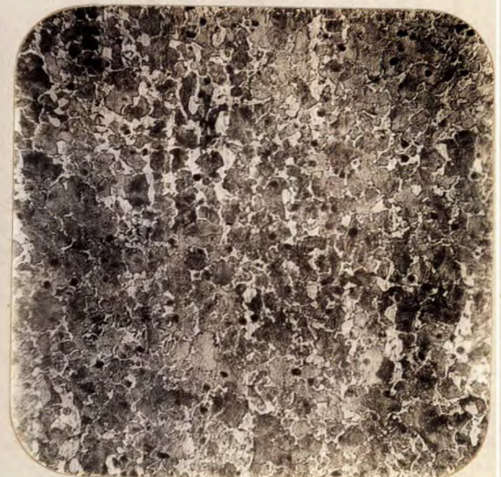
X100, nital etch. Grain size of 1 1/4"-diameter bar at 1700° F.
