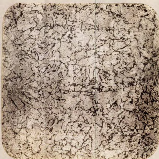
X100, HCl-picric acid etch. Grain size of 3 1/4"-diameter bar at 1550° F.
