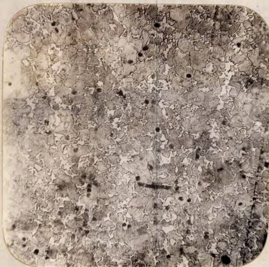
X100, nital etch. Grain size of 3 1/4"-diameter bar at 1700° F.
