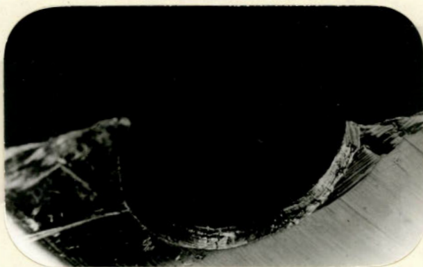
CHAMFER ON THE OIL HOLE. (Approximately X6 magnification).
