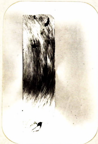
DEFECTS IN LINK NO. 2. (Approximately to size).
