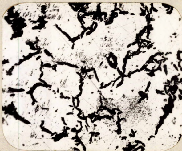
X100, nital etch. PRIMARY GRAPHITE AFTER ANNEALING.
