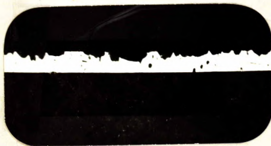
Magnification, X40. CROSS-SECTION OF CHROMIUM PLATE, SHOWING SURFACE IRREGULARITIES.
