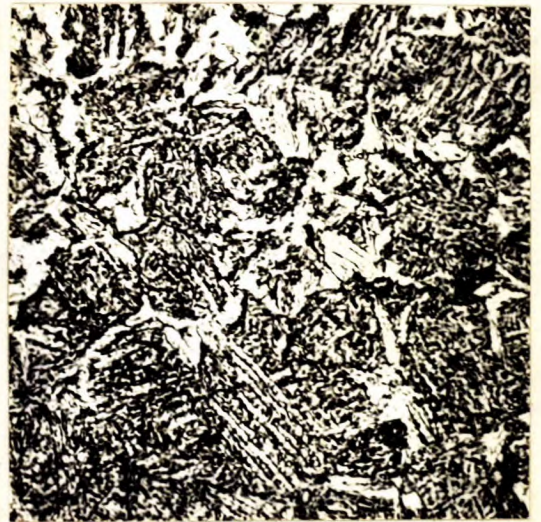
Photomicrograph, X1000. Electro polish, picral etch. Structure 1 inch below surface, resulting from controlled quench from 1500° F. and draw at 800° F. Note small amount of ferrite present. Compare with Figure 4.
