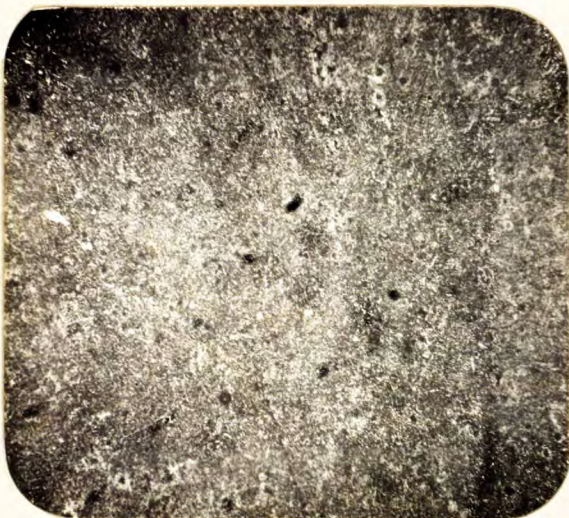
X100, nital etch. Sample "A" Sorbite.
