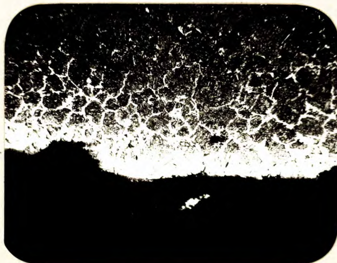
X100, nital etch. Sample "A" Above decarburized edge is typical of all springs examined.
