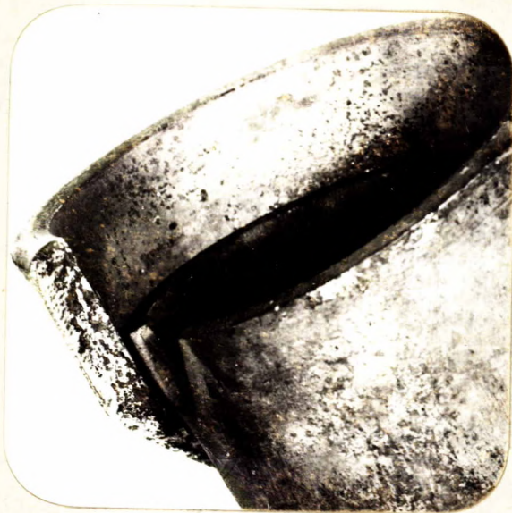
Fracture of Spring "D".
