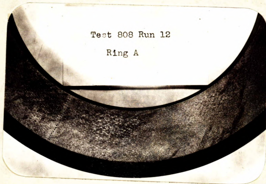
Segment of Ring A after the macro-etching (Approximately actual size).
