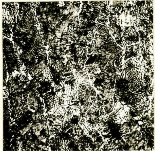
X2000, picral etch. AVERAGE STRUCTURE OF BROKEN BALL.
