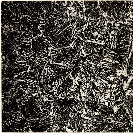
Photomicrograph, X500, picral etch. Note crack.
