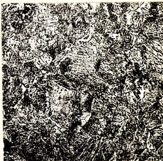
Photomicrograph, X500, picral etch.
