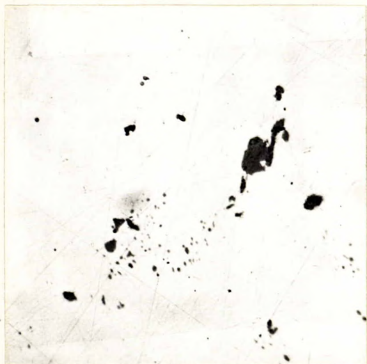
Photomicrograph, X250, polished to show inclusions.
