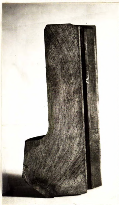
Macro-etch of section of hub of broken flange.
