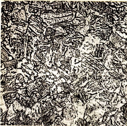
X500, nital etch. TYPICAL CORE.
