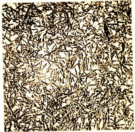
TYPICAL CASE X1000, nital etch.
