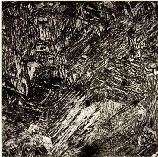
X500, nital etch. CORE OF PIN NO. 2. Figure 5.
