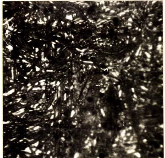
X1000, nital etch. CASE OF PIN NO. 2. Figure 6.
