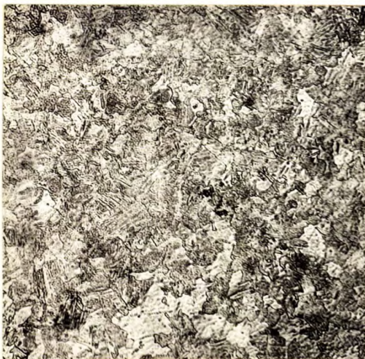
X500, nital etch. CORE OF CANADIAN ACME PIN. Figure 3.
