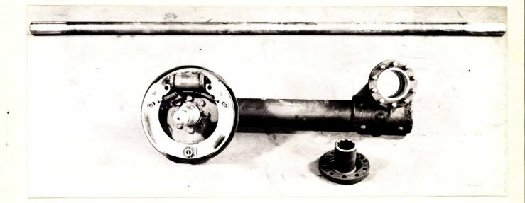
SUBMITTED PARTS OF BOAT TRAILER WHEEL SPRINGING MECHANISM.
