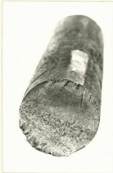
FATIGUE FRACTURE (Approximately to size).
