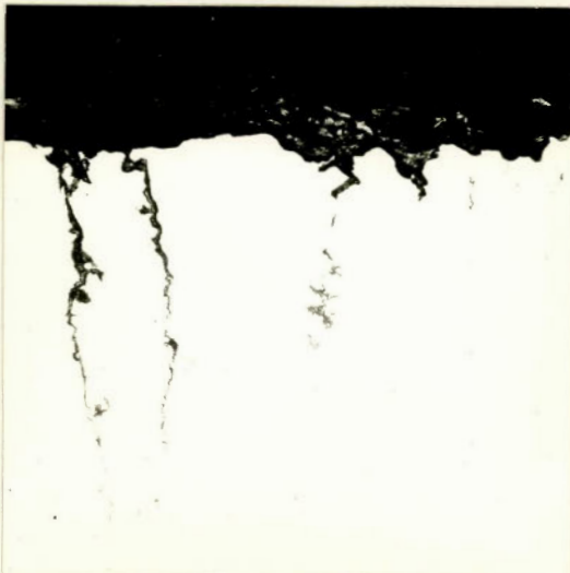
X100, unetched. CORROSION FATIGUE CRACK.
