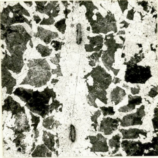
X100, picral etch. PHOTOMICROGRAPH OF LONGITUDINAL SECTION.
