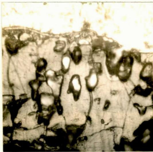
Photomicrograph, X1000, of slag found on metal- weld interface.
