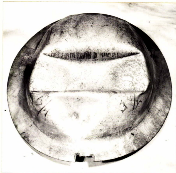
Standard manganese steel helmet deformed by falling onto a two-inch channel iron with 1,305 foot pounds energy.
