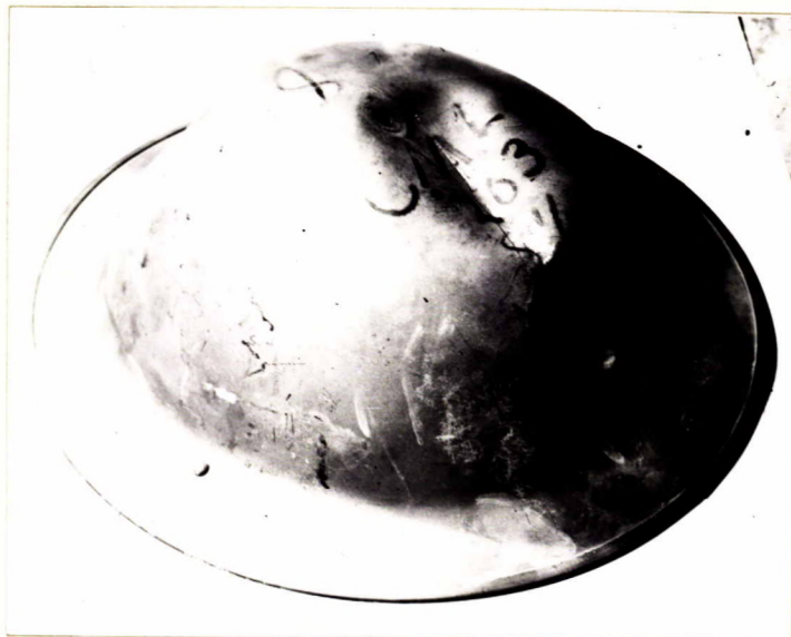
Standard manganese steel army helmet deformed by a brick falling from a height of 17 feet.
