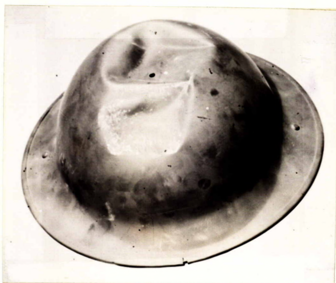
Steel helmet deformed by a brick falling from a height of 34 feet.
