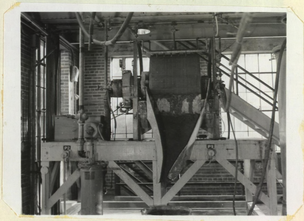
Oliver filter, filtering aluminate solution from dicalcium silicate residue.
