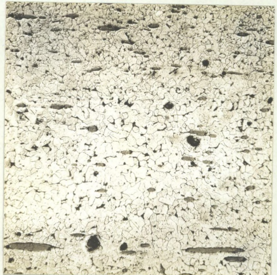
X100, picral etch. MICROSTRUCTURE AFTER NORMALIZING.
