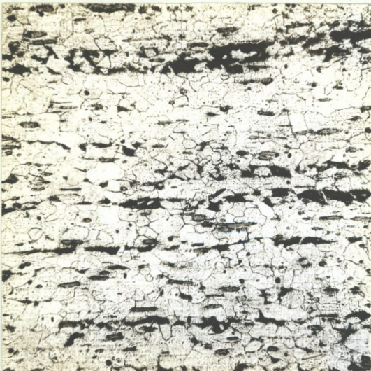
X100, picral etch. MICROSTRUCTURE AS RECEIVED.
