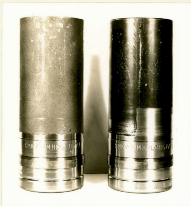
Photograph showing apparent eccentricity of machining.
