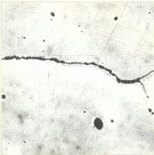
X200, picral etch. GENERAL STRUCTURE OF METAL. (Note small crack on grain boundary.)
