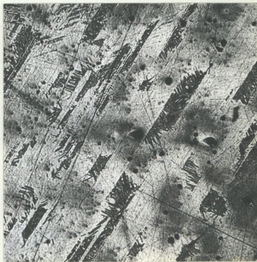
X200, picral etch. CONDITION OF METAL IN VICINITY OF WIDE CRACKS.
