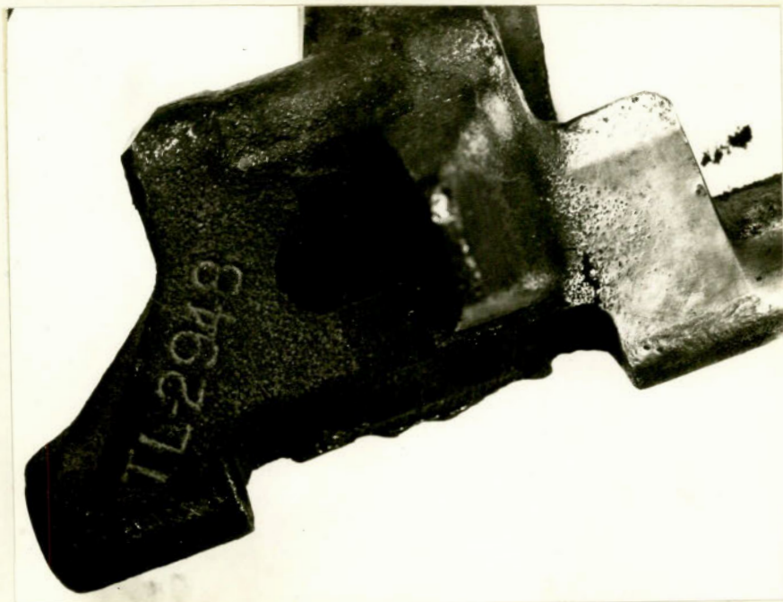
CRACK REVEALED BY MAGNAFLUX.
