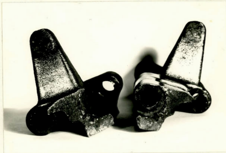
APPEARANCE OF FRACTURED CASTING.
