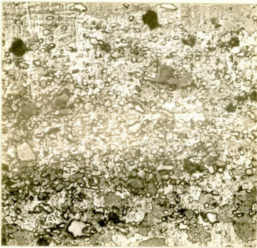
X250, etched with Keller's reagent.®
