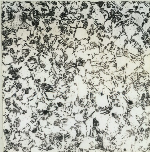
X250, nital etch. CORE OF PIN F. (C.P.R., 410 miles)
