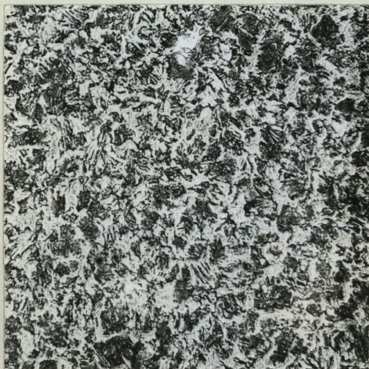
X250, nital etch. CORE OF PIN B. (C.P.R., no mileage)
