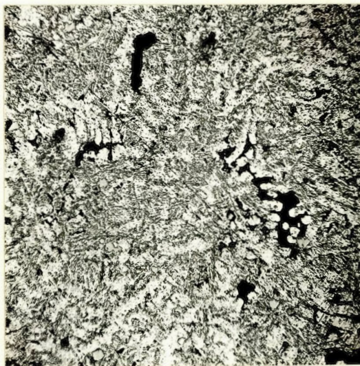
X100, unetched. Section in weld area.
