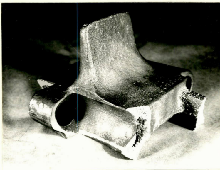
Shrinkage Cavity at Fracture. (Approximately \frac{1}{2} size)
