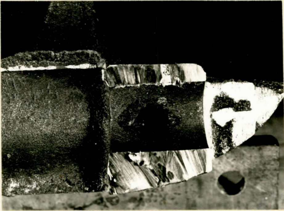
Flaw on End of Bearing Hole. (Approximately to size)
