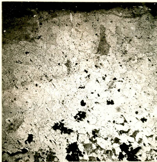
X100, nital etch. Decarburized area of bottom link.
