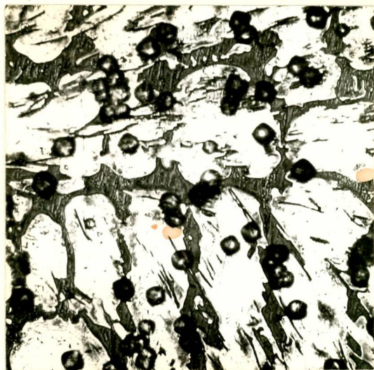
X500, Murakami's reagent etch. White cast iron.
