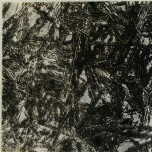
X1500, Nital etch. Core of hot-quenched link.
