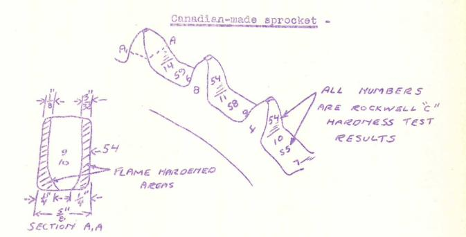
SECTION THROUGH SPROCKET TOOTH
