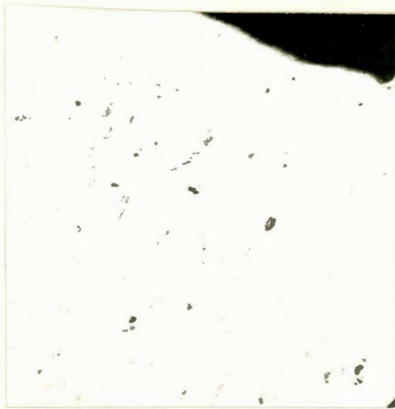
Dirt inclusions in steel. x100, unetched.
