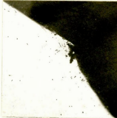
Edge of fracture. x100, unetched.
