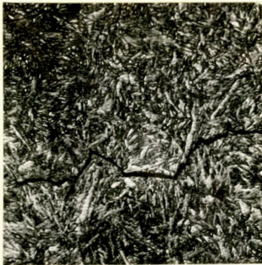
X1000. Case Structure, Showing Crack.
