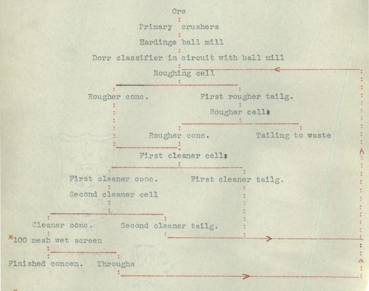
Note: It may be advisable to dispense with the 100 mesh wet screen as this ore contains very little impurities, such as iron pyrites, an a high grade concentrate should be produced without the addition of the screen.
