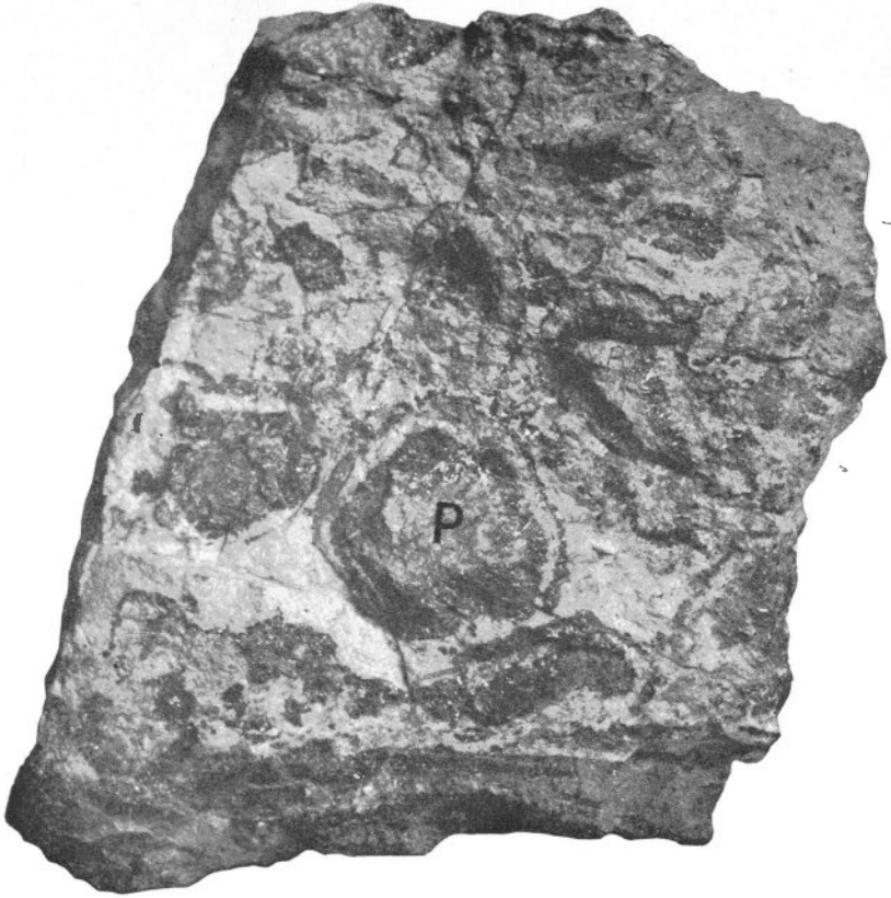
ILLUSTRATION OF CRUSTIFICATION AND THE ORDER OF MINERAL DEPOSITION IN THE HIGHLANDER VEIN.
