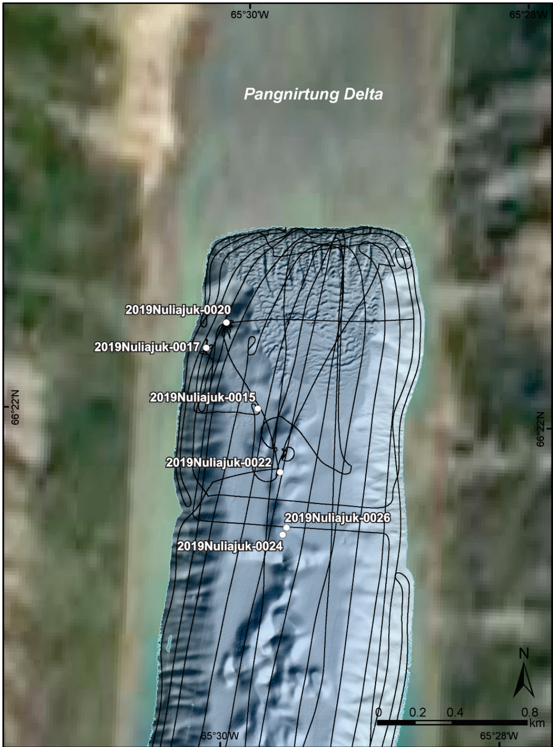
Figure B18: Location of cores 0015 to 0026 and 3.5 kHz sub-bottom profiles collected in Pangnirtung Fjord
