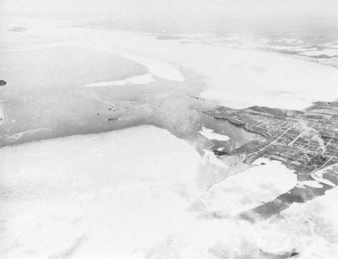
Figure 45. Decayed winter ice, drifting past Dalhousie is no obstacle to the freighter anchored in mid-channel; however, in Chaleur Bay the ice fields were congested for freighters without icebreaker support. (Alt. 5,000 feet, April 27, 1961).
