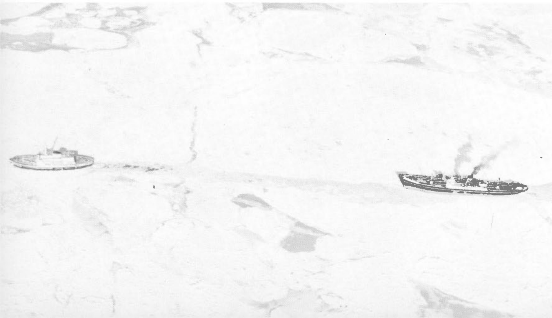
Figure 46. Severe pressure in icefields 4 to 5 feet thick causes the wake of the icebreaker C.M.S. John A. MacDonald to close rapidly and restrict progress of the freighter following (Feb. 2, 1961).
