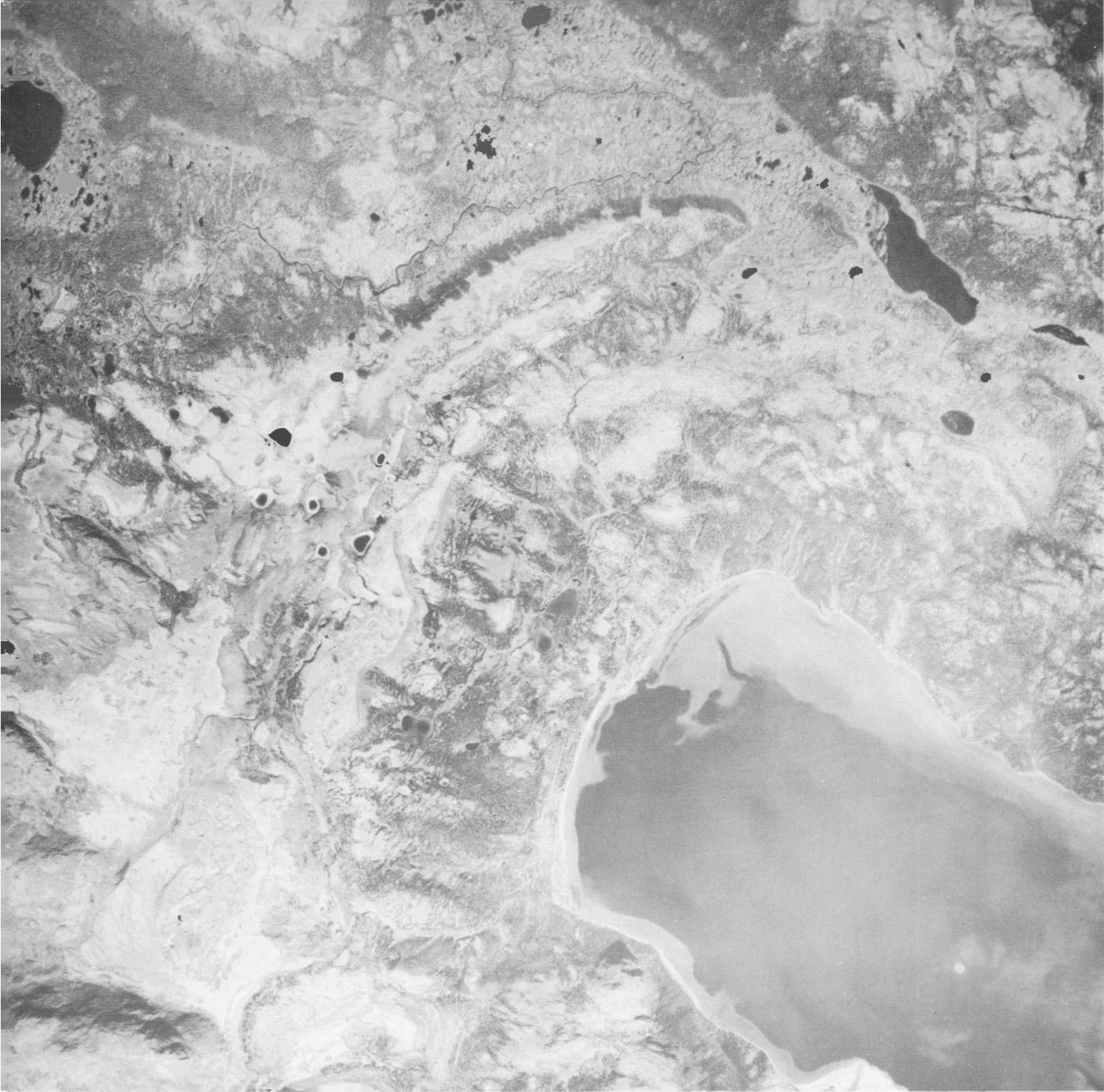
Figure 8. Vertical airphoto showing the western end of Lake Tasiuyak Tasiyua from 21,000 feet. Part of the main end moraine system roughly parallels the lake shoreline. Outwash deposits and numerous large kettle holes can be seen. (RCAF Photo).
