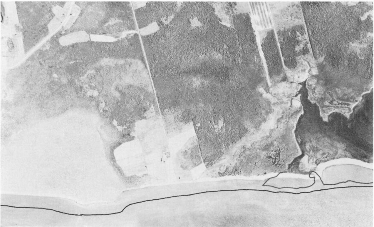
Figures 6 and 7. This rapidly eroding section is composed of a peat exposure 4 to 7 feet in height on the left and a low bank of unconsolidated material on the right. Along the base of the erosion face at left, wave action has exposed a tangled mass of tree stumps that had been covered by several feet of peat. The sea is now encroaching on the cultivated land (centre), and is threatening the nearest house with inundation in a few years' time.
