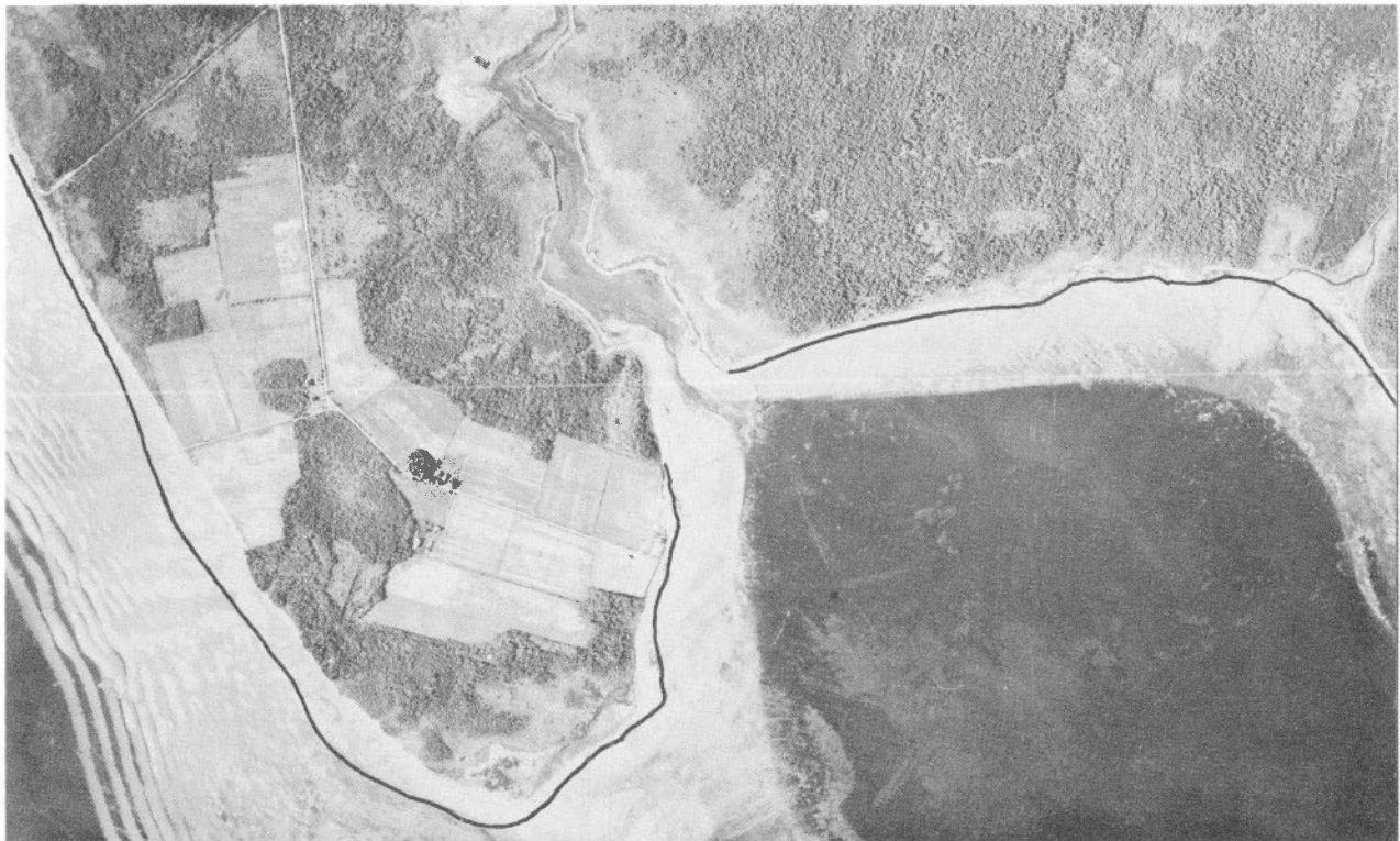
Figures 19 and 20. Miscouche Point has experienced a most alarming loss of land. On the west side of the peninsula the rate of retreat reaches nearly 13 feet per year at some points. The erosion face, of unconsolidated material, varies in height from 2 to 5 feet. During the brief span of 23 years large parts of several cultivated fields have been removed and the acreages of the farms considerably reduced.
