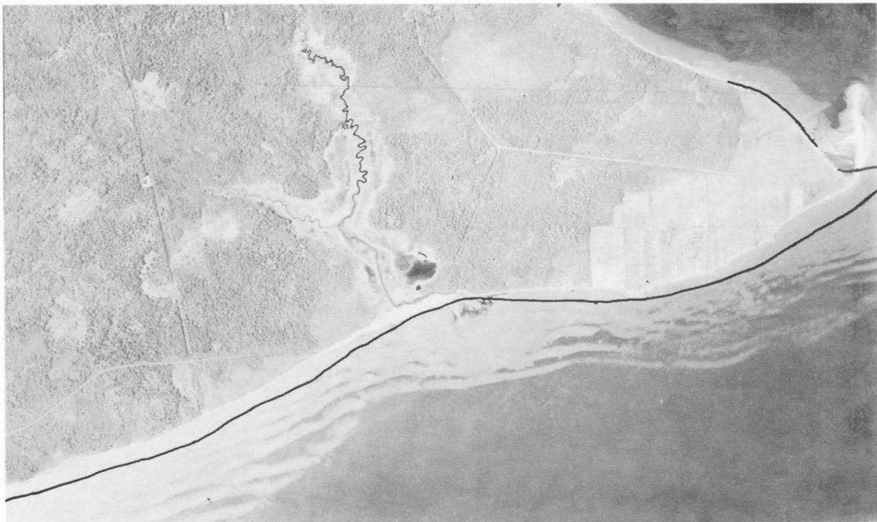
Figures 17 and 18. Sunbury Point is a remarkable example of rapid shoreline retreat. Except for a short section of rock, the coastline is of unconsolidated material. The rate of retreat varies, being slightly lower where the rock offers greater resistance and where deposition has occurred at the stream mouth. Shoreline retreat on the north side of the peninsula has been far less severe. The cusped bar at the end of the point has turned north and taken the form of a spit.
