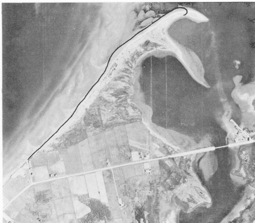
Figures 14 and 15. Successive sand ridges show that this compound, recurved spit has been altered in shape frequently. Since 1935 rapid erosion has occurred on the seaward side and the secondary point of the spit has curved landward. Only the primary recurved point existed in 1839, as indicated by the Bayfield survey.
