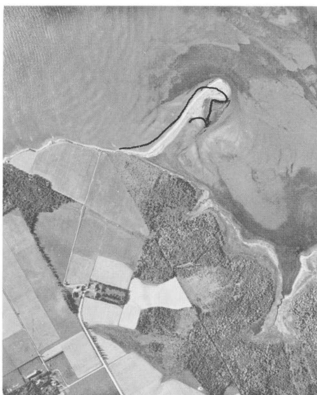
Figures 23 and 24. Situated on the opposite side of Salutation Cove is a spit which was formerly of much greater size. The 1839 chart shows a substantial sand feature that reached almost to the northern shore of the bay, constituting a baymouth bar. Since 1935 the spit has lengthened and become more attenuated.
