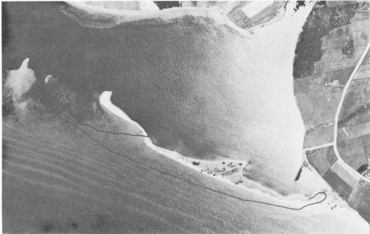
Figures 10 and 11. During the 23-year interval a large part of the bar has been sliced away and sand has been deposited in abundance at the eastern end, joining the bar to the land. That this bar was once much larger is indicated on the 1839 Admiralty chart (Figure 2). At top right, the fact that the barn situated on the point is much closer to the water in Figure 11 than in Figure 10 is evidence of shoreline retreat.
