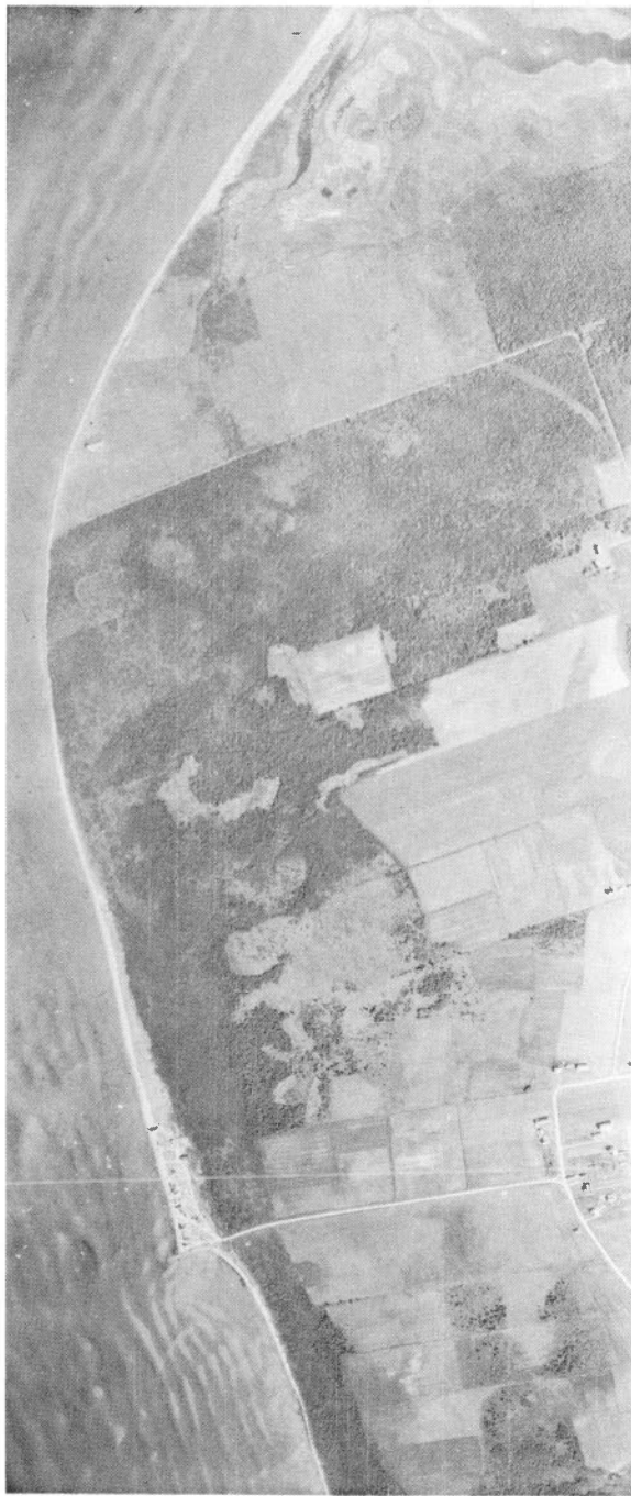
Figures 12 and 13. The coast near St. Chrysostom is composed of unconsolidated material and the erosion face ranges from 2 to 5 feet in elevation. The shoreline has retreated at a rate of approximately 5 feet per year. Sand that had accumulated north of the wharf before 1935 was eroded away during the succeeding quarter century.
