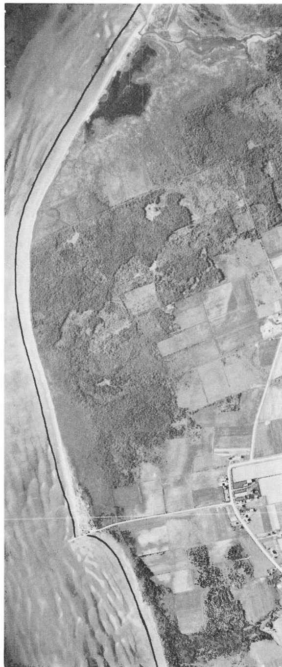
Figures 12 and 13. The coast near St. Chrysostom is composed of unconsolidated material and the erosion face ranges from 2 to 5 feet in elevation. The shoreline has retreated at a rate of approximately 5 feet per year. Sand that had accumulated north of the wharf before 1935 was eroded away during the succeeding quarter century.
