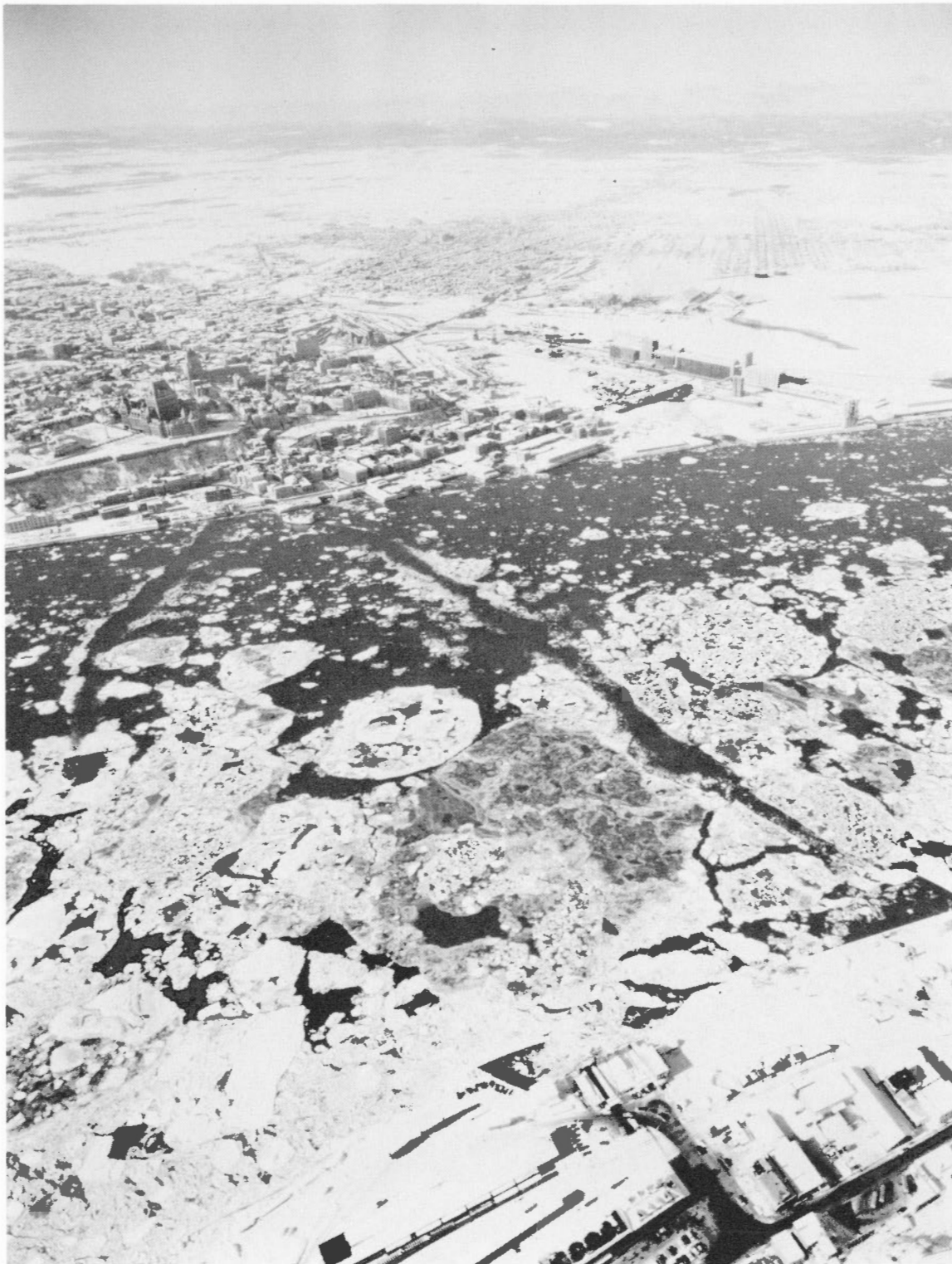
Figure 62. The ice on the St. Lawrence River at Quebec on January 27 consisted mainly of new and young ice types intermixed with small floes of winter ice that had broken from the edge of the shorefast ice. (Alt. 2,900 feet)
