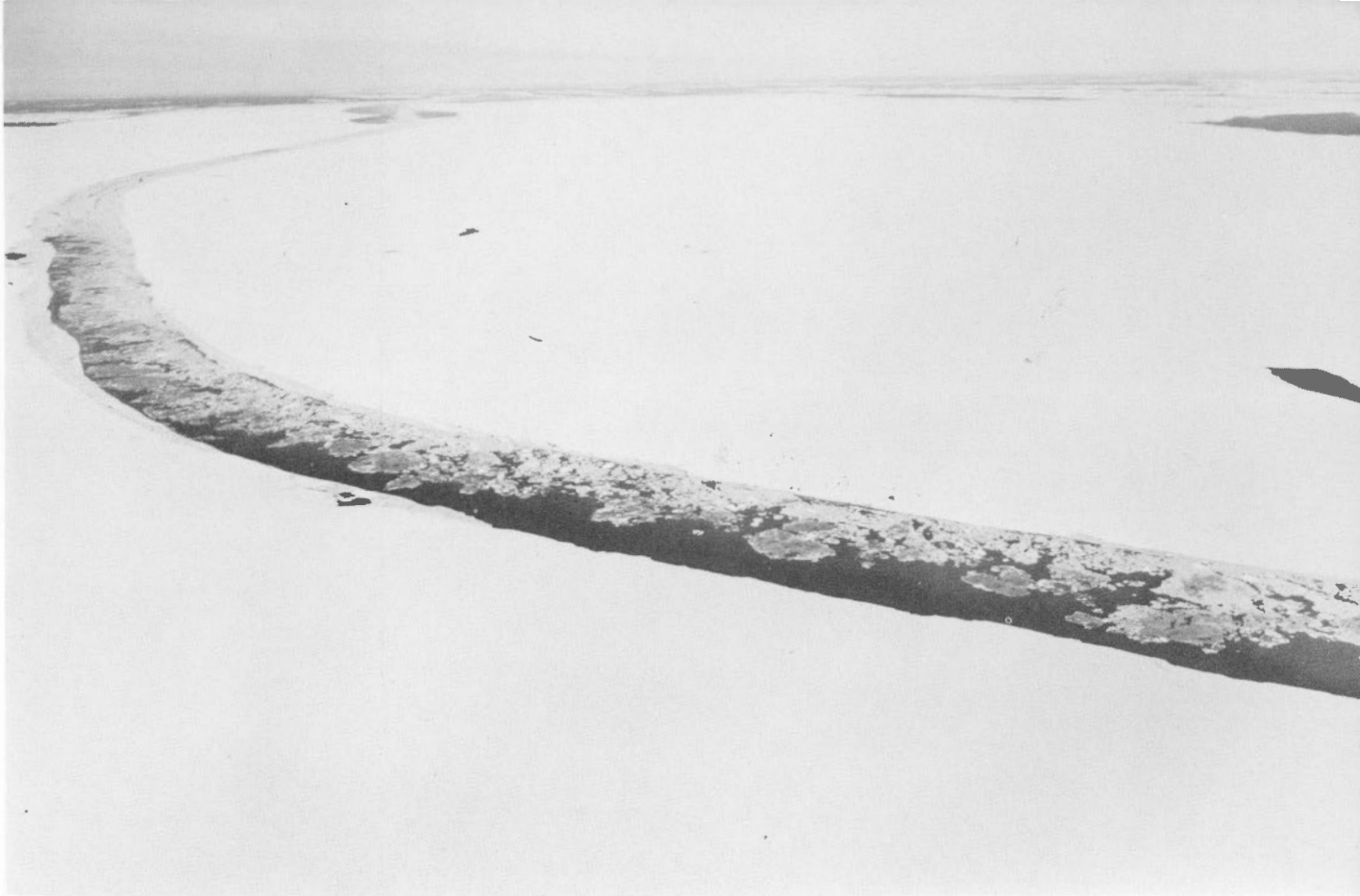
Figure 58. Congestion and consolidation of the ice in the Lake St. Peter reach of the river begins early and ends late. The main problem for the icebreaker in this area is to keep the ice moving downstream. (Alt. 1,600 feet, Mar. 1, 1960)
