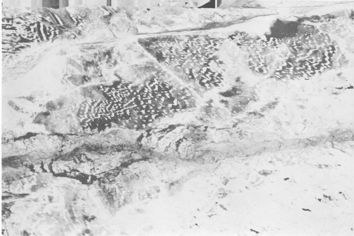
Figure 35. A landfast field of new and young ice, with winter ice in the lower right. The disturbance in the ice is caused by the passage of an icebreaker. (St. Lawrence River near Sorel, alt. 1,100 feet, Jan. 6, 1960)
