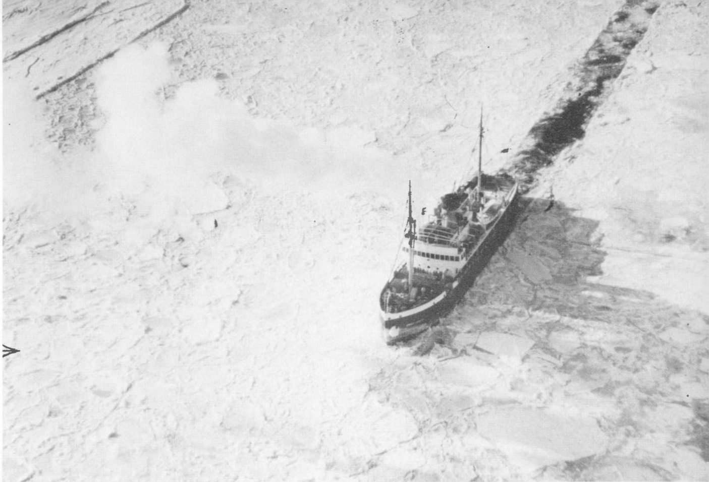
Figure 36. (February 20, 1959). The ship channel in the St. Lawrence in winter is clearly marked as it lies between the encroaching edges of landfast ice. During prolonged cold periods, the floating ice in the channel anchors to the landfast ice, consolidates, and may become a considerable barrier for an icebreaker to crush. The C.G.S. Ernest Lapointe is pushing up-river in the vicinity of Verchères. (Altitude 500 feet).
