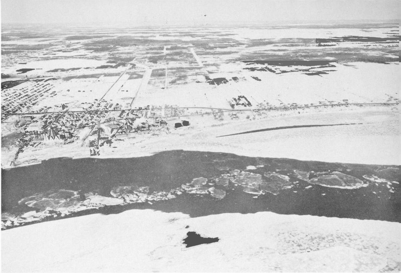
Figure 40. (March 5, 1959). The ship channel at Three Rivers is bordered by landfast ice. Winter ice broken from the edge of the landfast ice is usually an important constituent of the ice in the ship channel. (Altitude 1,900 feet).
