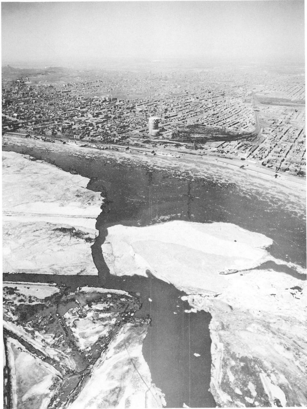
Figure 51. (April 14, 1959). The icebreaker C.G.S. Ernest Lapointe is in the process of breaking up a mass of landfast ice that is blocking the eastern entrance to the Seaway canal at Montreal. The ice drifting downstream on the north side of the river provided no obstacles to the freighters that have docked along the Montreal harbour front. (Altitude 1,700 feet).
