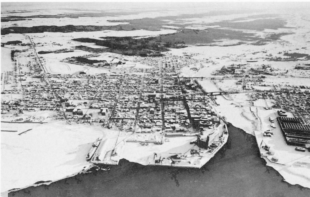
Figure 26. (January 23, 1959). Landfast ice on the south shore converges on the port of Sorel, freezing in the shipping. The mouth of the Richelieu River is kept relatively ice-free by frequent ferry crossings. (Altitude 1,800 feet).
