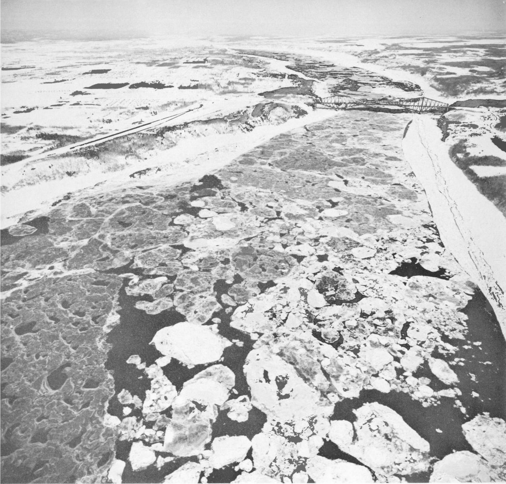
The shores of the St. Lawrence River converging toward the Quebec bridge, provide a funnel effect, constricting the ice as it passes under the bridge. This is an area of frequent ice jams. Landfast ice, bordered by massive pressure ridges, extends from the shores. Ice coverage of above 9/10 consists of new, young and winter ice forms. (Altitude 1,800 feet, March 8, 1959).
