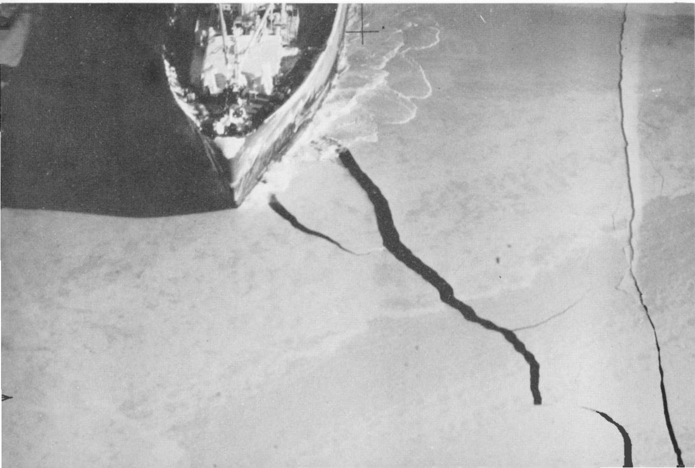
Figure 32. (February 12, 1959). The Danish ship, Helga Dan , passing through young ice near Seven Islands, shows no accumulation of ice about the bow. This ice consisting formerly of very young ice has been subjected to intensive shelving. The ice is grey and opaque, and the cracks in it are sharp. (Altitude 600 feet).
