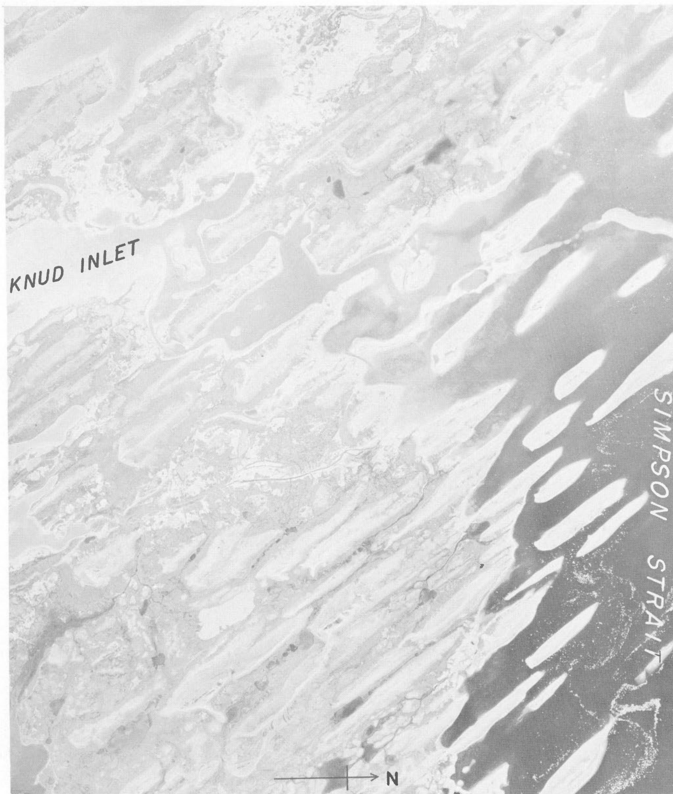
Figure 8. Knud Inlet area, Adelaide Peninsula; a vertical photograph taken at 30,000 feet showing the drumlin field oriented northwest-southeast. Two eskers flank the inlet, and localized marine plains appear as light-toned mottled areas to the left. Strands occur on the drumlins.
