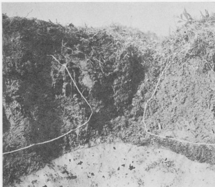
Figure 5. The white string marks the boundary between mineral soil and organic material. An ice-wedge shows up as white in the bottom of the photograph. Note how organic material occupies the depression. Permafrost is 12 to 18 inches below the surface.
