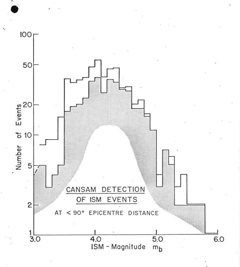
Figure 2. Automatic detection of ISM events by CANSAM system. ISM Background is also  $\checkmark$  90  $^{\rm O}$  from YKA
