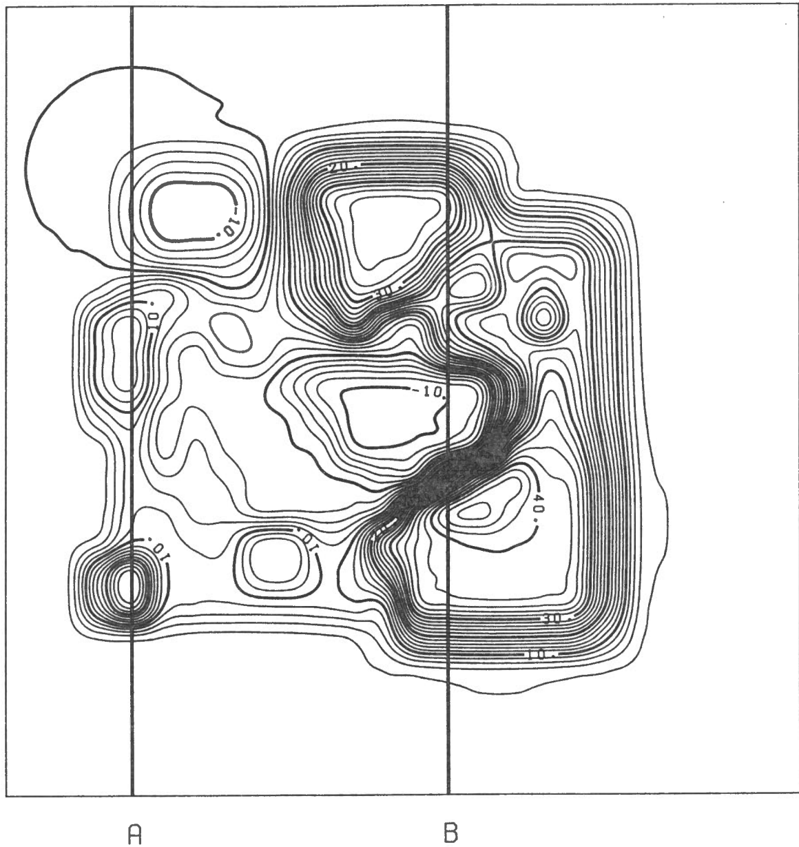
Figure 4 Contoured Gravity Over a Region Located in Northern Ontario (Nagy, 1986). Profiles A and B were selected from this region and used as input for the gravity filter described in the text. The margins of this figure define an area of 125 x 125 km.
